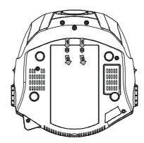
2.) Insert 6 pcs "C" size batteries into the battery compartment according to the polarity diagram engraved inside the compartment. If the batteries are inserted incorrectly the unit will not work.
